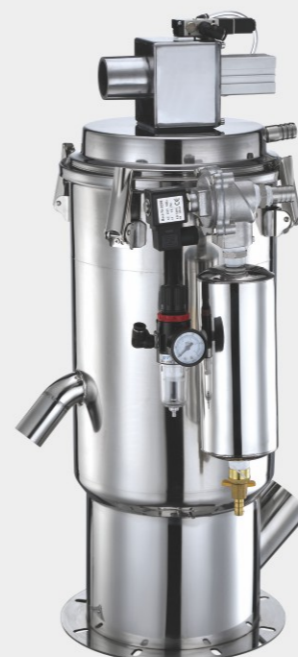
除尘料斗 Dust removal hopper
