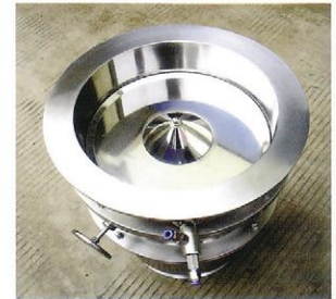
Side spraying for pellet and coating
