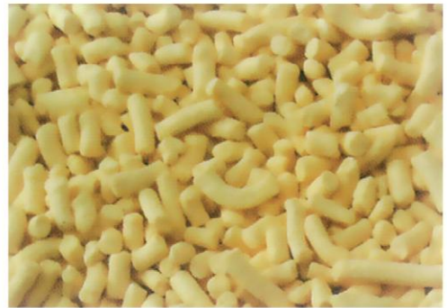
Granules after drying by vibrating fluid bed dryer
