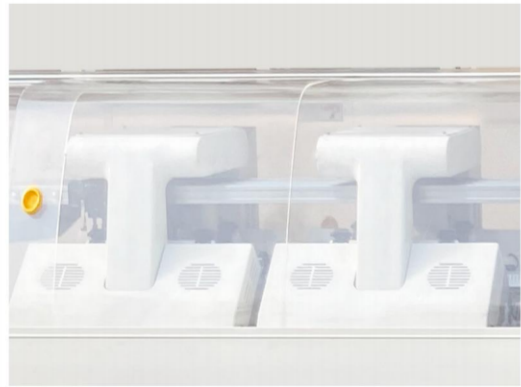
双系统双机头，最长可达120英寸。根据织物宽幅，编织宽幅时机头合并为四系统，编织窄宽幅时机头分开，二个机头同时编织二个织物。 Double system double carriages, up to 120 inch. According to the width of the fabric, when knitting wide fabric, machine carriages will be combined into four system. When knitting narrow fabric, machine carriages will be separated.
