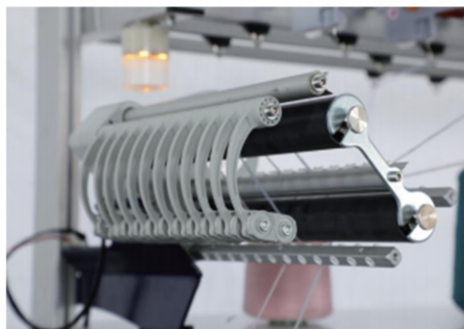
送纱装置，多股进纱减小阻力，进纱张力均匀。增加防缠绕装置有效解决纱线缠绕烦恼。 Yarn feeding device, multi strand feeding to reduce resistance, and uniform feeding tension. With anti-winding device to effectively reduce yarn winding.
