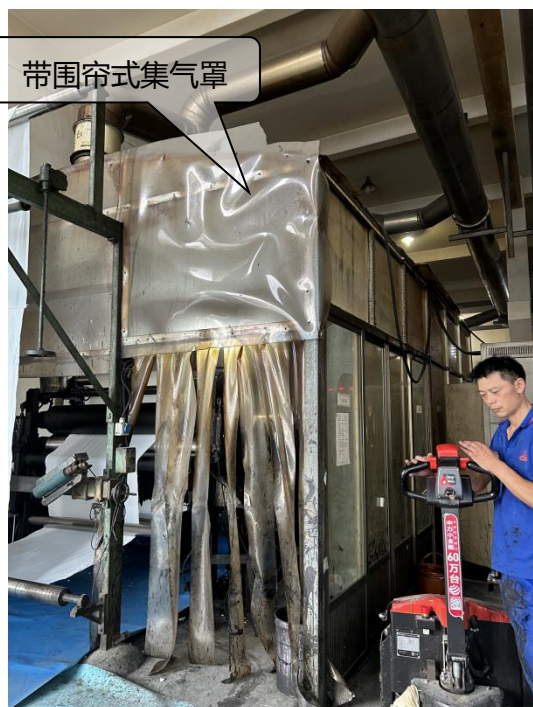
涂布废气带围帘式集气罩收集
