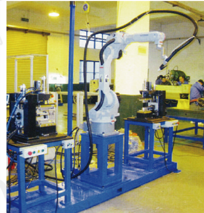
• Frame robot welding unit
