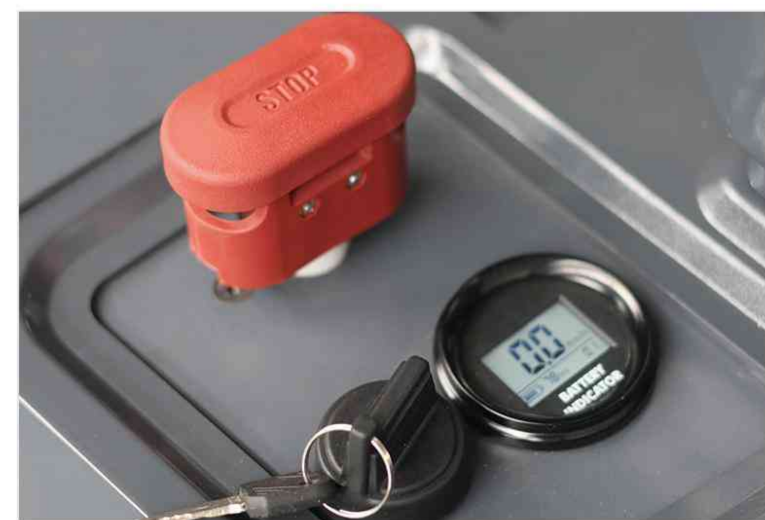
Emergency switch Battery indicator
