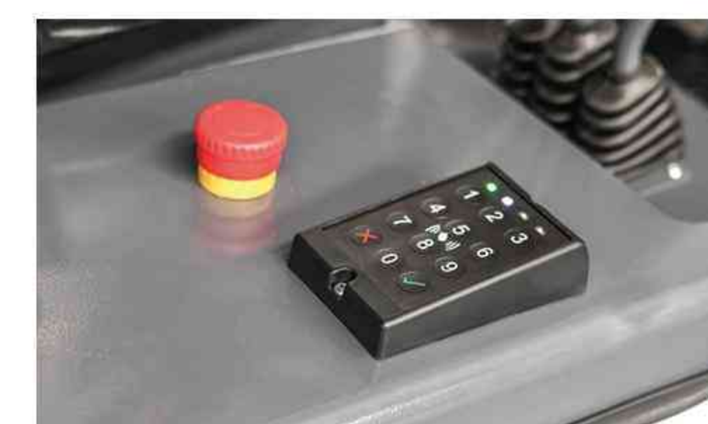
Emergency switch + Pin-code lock
