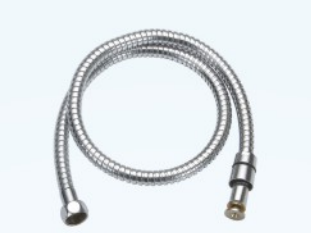
YSA011 360°旋转不锈钢双扣管 YSA011 360°rotary double-buckle stainless steel pipe 直径 Diameter Ø14mm 规格 Specification F1/2xF1/2x(1.2-2m)
