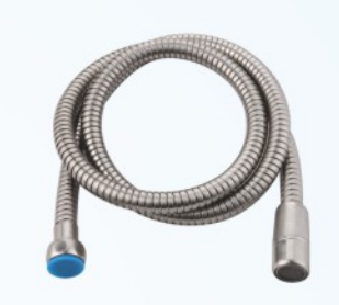
YSA015 镍拉丝双扣管 YSA015 Nickel wire hose double-lock 直径 Diameter Ø14mm 规格 Specification F1/2xF1/2x1.5m
