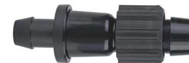
No.:56216BS(1600) Applicable water pressure 1.5-3.5Kpa flow 1600L/H Φ 20 Off take ( Pressure compensating )
