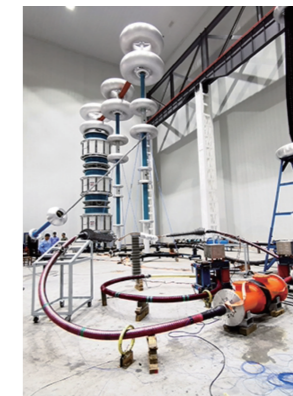
110kV电缆快速恢复接头型式试验 Type Test for 110kV Cable Quick Recovery Joints
