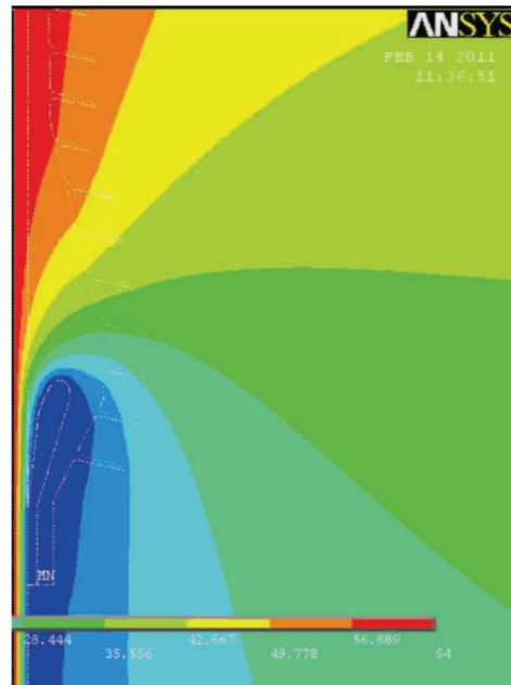
预制电缆终端电场分布 Electric Field Distribution of Pre-molded Cable Terminations
